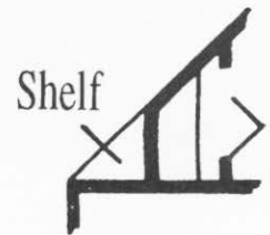
PLANT SELF DETAIL AT CORRIDOR TO KITCHEN
